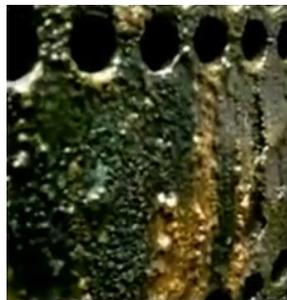
Microbiological induced corrosion at end of tube sheet in chiller
