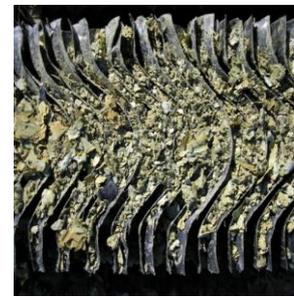
Scaling in the fill of a cooling tower, due to low inhibitor rates and high conductivity.
